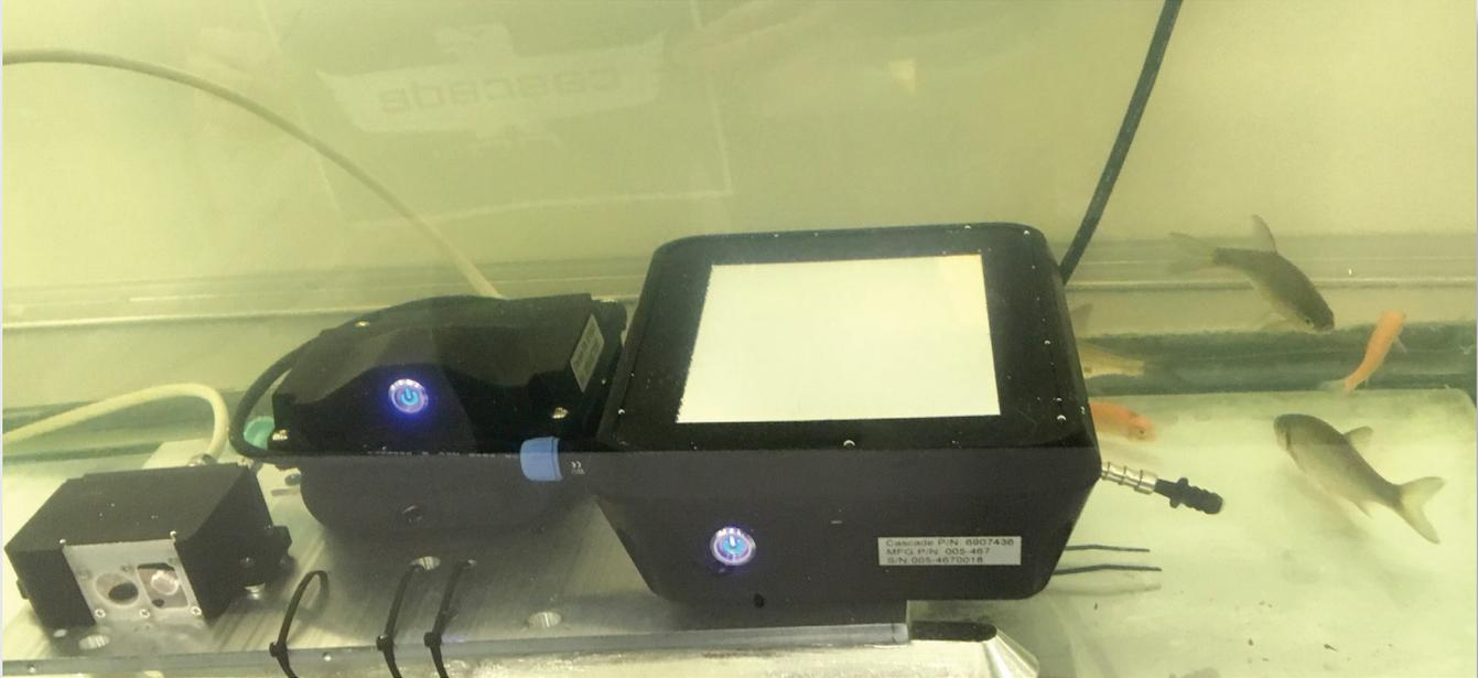
*SensorForks camera system submerged in water to test against the IP67 standard for water ingress.*
